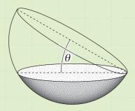
( $\alpha$ ) Find  $\theta$  so that the depth of water remaining is one half of the original depth.
